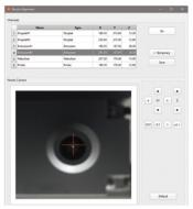
• By automatically recognizing the surface height value of bioware and fine-tuning the X / Y coordinates between the nozzles used for output, highly stable extrusion 3D Printing can be achieved.
